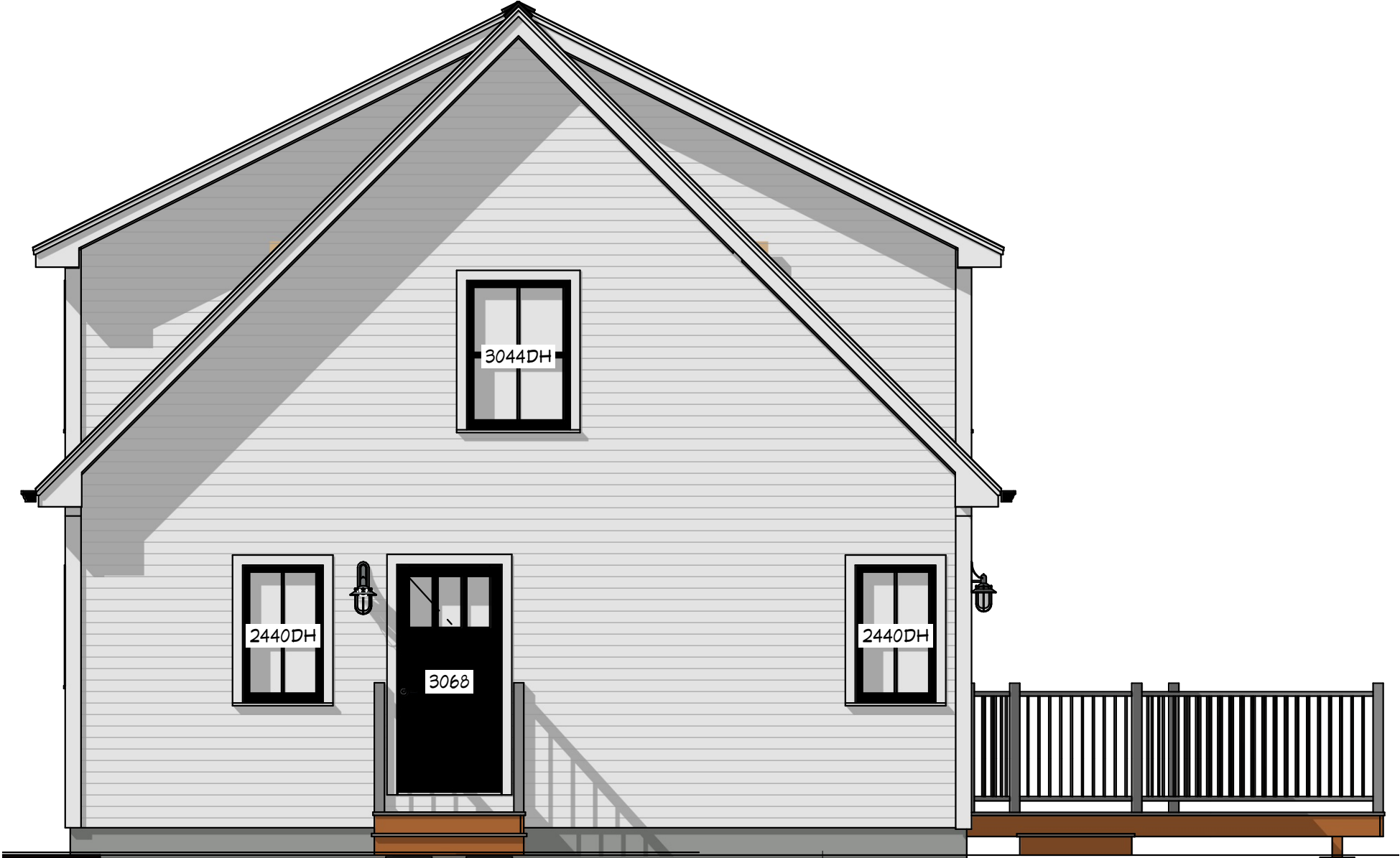
Exterior Elevation Right 1/4 in = 1 ft
