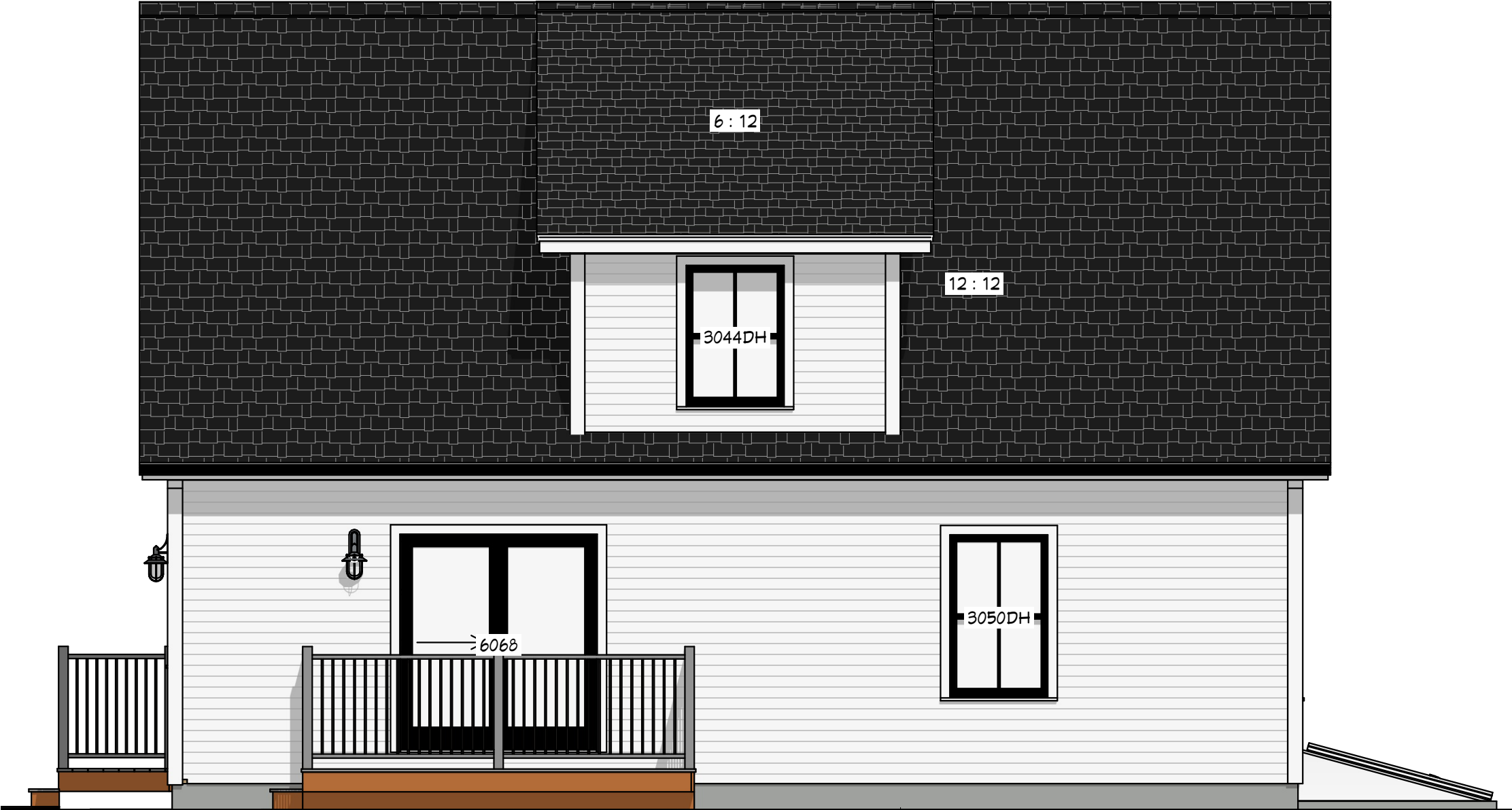
Exterior Elevation Back 1/4 in = 1 ft
