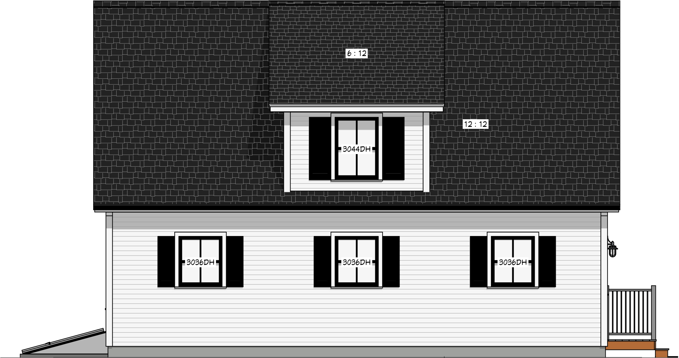
Exterior Elevation Front 1/4 in = 1 ft
